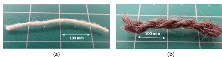
Figure 1. Yarns of the fibres used on the composites—(a) Sheep's wool yarn; (b) Dog wool yarn.
