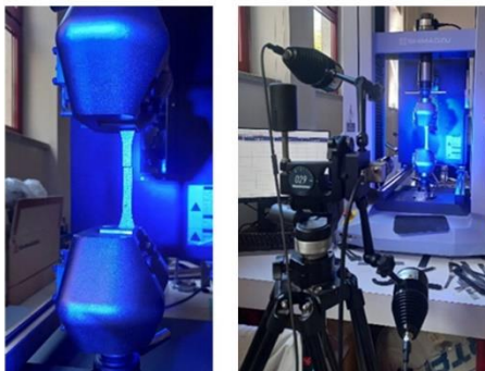
Figure 7. Tensile test and Digital Image Correlation setup.
