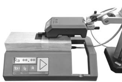
Figure 55 – Hommel T1000 linear surface profiler and LV16 unit.
