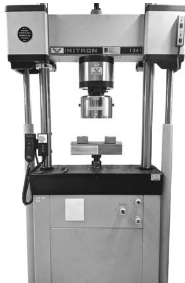
Figure 51 – Instron 1341 testing machine.
