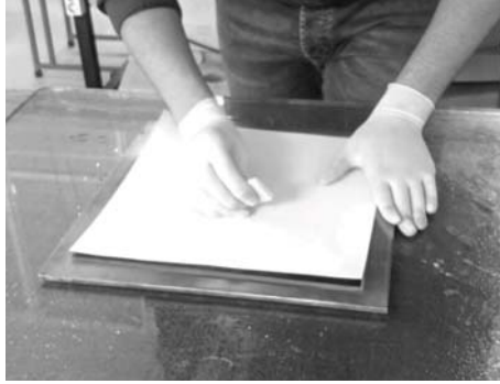
Figure 38 – Application of hand pressure during layup.
