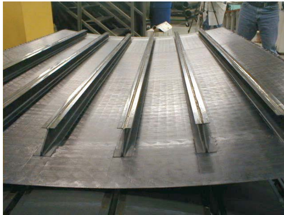
Figure 3 – Composite (Carbon fibre/PEEK) skin panel with co-bonded T-stiffeners [11].
