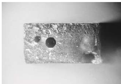
Figure 31 – Typical fracture surface of the bulk adhesive.
