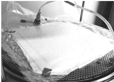
Figure 39 – Bagging setup for curing the CFRP laminate.
