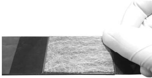
Figure 59 – Application of a fibreglass veil as a carrier for the adhesive.
