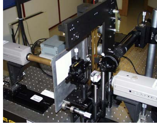
Fig. 3. Experimental optical apparatus for retro-diffusion and transmission analysis.
