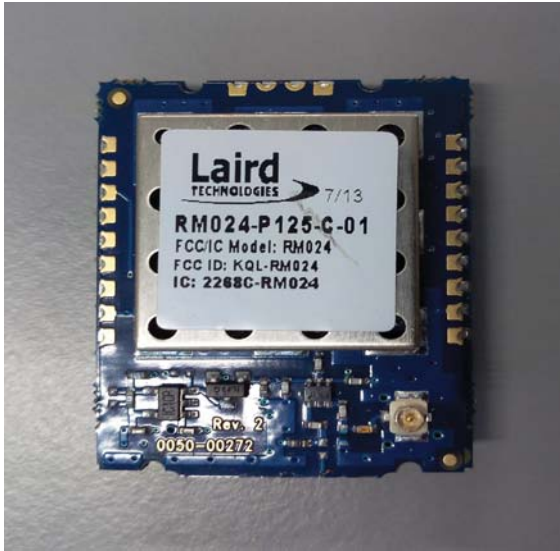
Figure 6.7: Laird LT2510 RM024-P125-C-01 (125mw power version). Figure 6.8: Oracle video diversity controller used to bridge two video receivers.
