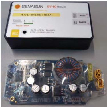
Figure 6.3: Genasun GV10-Li-12.5V MPPT controller with heat-shrink tubing.
