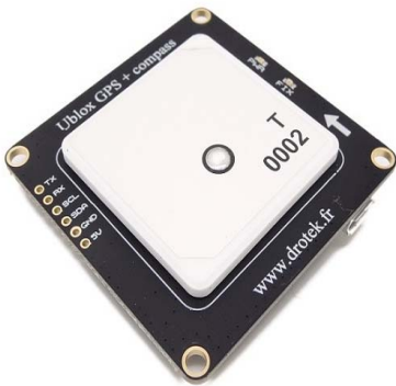
Figure 6.2: Ublox NEO-M8N GPS + HMC5983 magnetometer module (XL).
