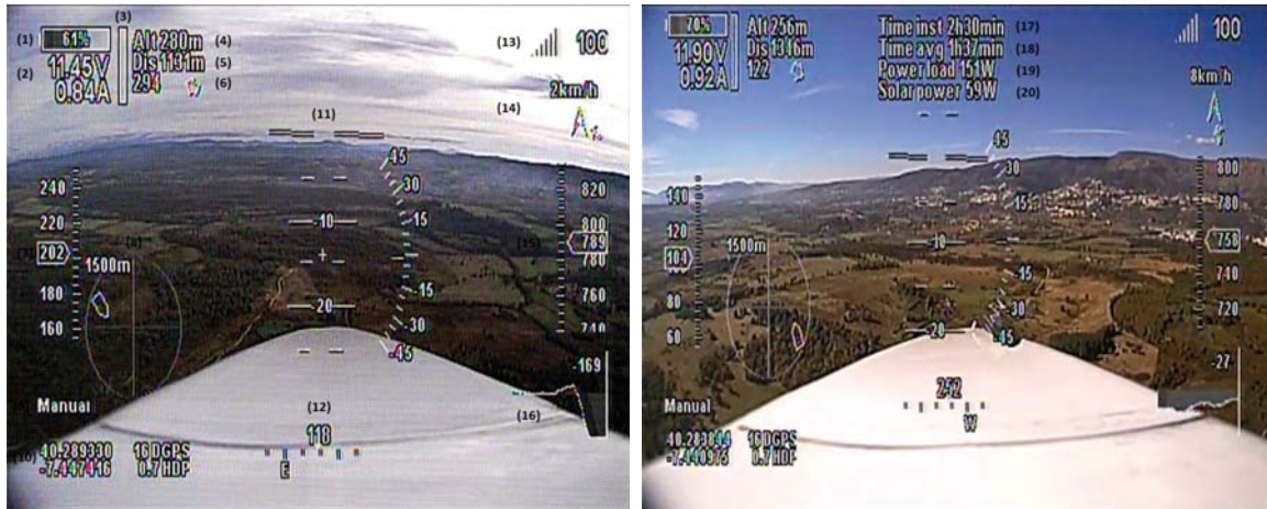
(a) Long endurance flight without solar panels using an AlceOSD (standard configuration). (b) Long endurance flight with solar panels using an AlceOSD (custom configuration)
