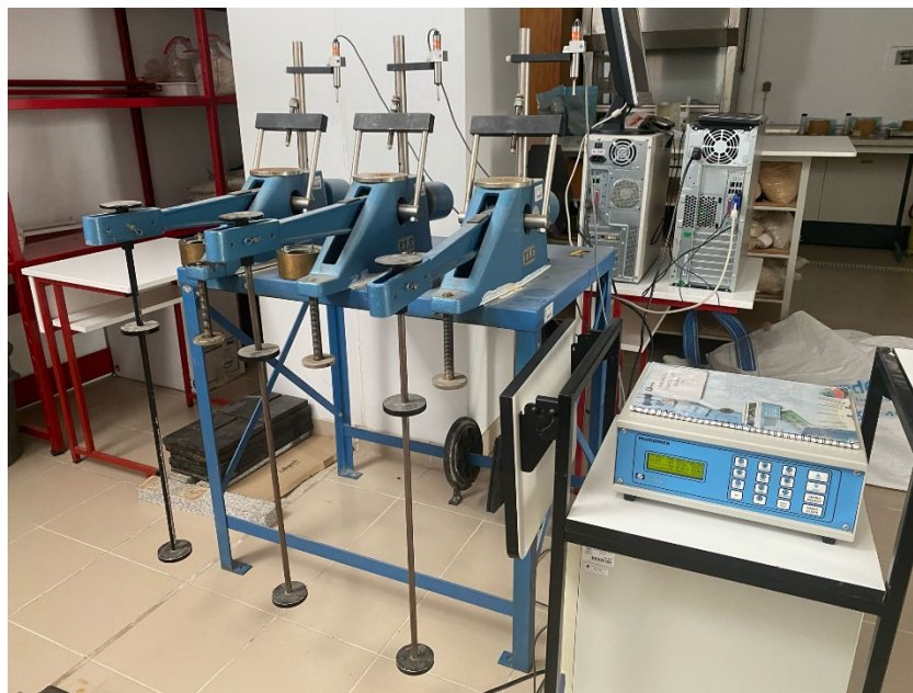
Figure 25 - Equipment used for the oedometric test (author)
