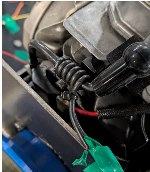
Figure 3.36: Tachometer cabled looped around the spark plug cable
