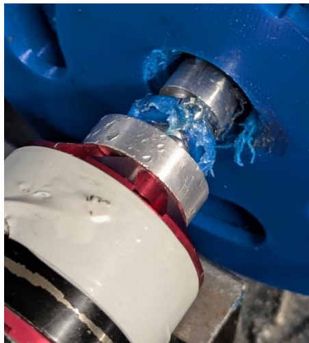
Figure 4.6: Remains of the holding ring
