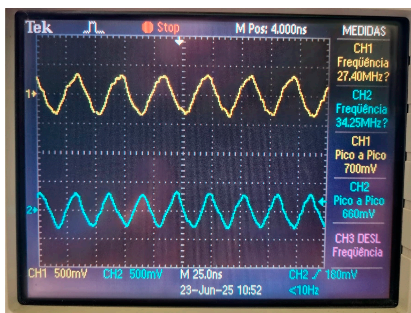
Figure 9. Clock line oscilloscope snapshot: Pixel Clock (yellow) and External Clock (blue).
