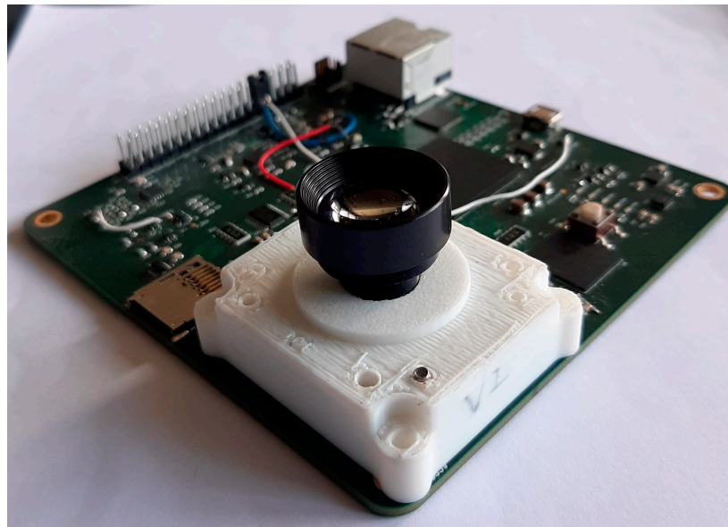
Figure 8. Final assembly of the STR miniature instrument.
