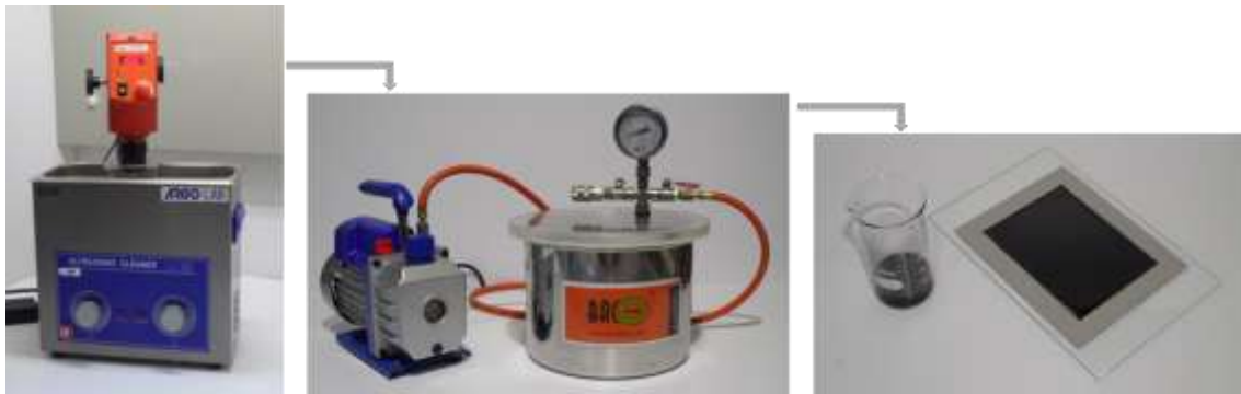
Figure 5.1: Methodology used to produce the nano-enhanced resins with CNFs.
