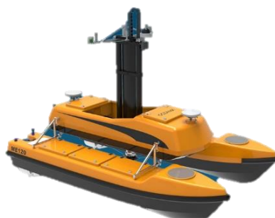
Figura 39: Hydrographic Unmanned Surface Vehicle ME120 (Oceanalpha, 2019)
