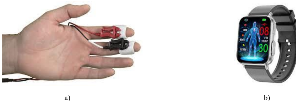
Figure 3.a) To detect electrodermal activity, electrodes are usually placed on the palms of the hands or the tips of the fingers, where there is a higher concentration of sweat glands. b) Example of a smartwatch that will be used to receive the data collected.
