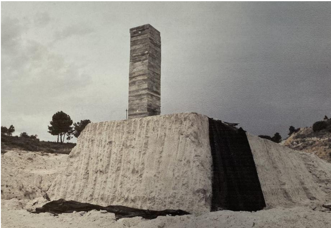
Figure 29. Plate load test
