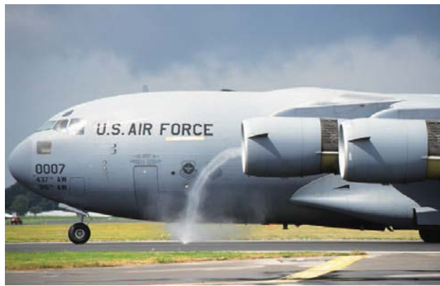
Figure 31: Ground vortex ingestion under reverse thrust operation.
