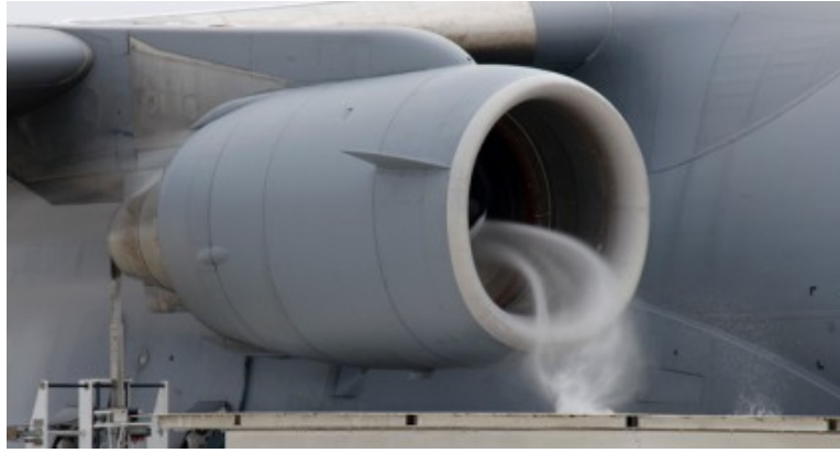
Figure 3: Ground vortex on a military turbofan engine visible due to water condensation inside core
