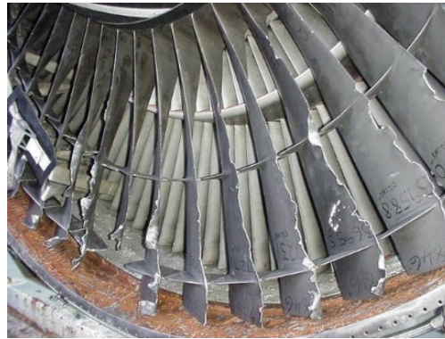
Figure 2: Effect of foreign objects damage (FOD) through ingestion.
