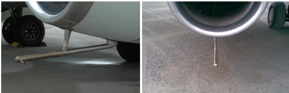
Figure 38: Vortex dissipater and gravel kit engine bleed air down and aft from 3 nozzles at the tip to break up the vortices in a Boeing 737-200.
