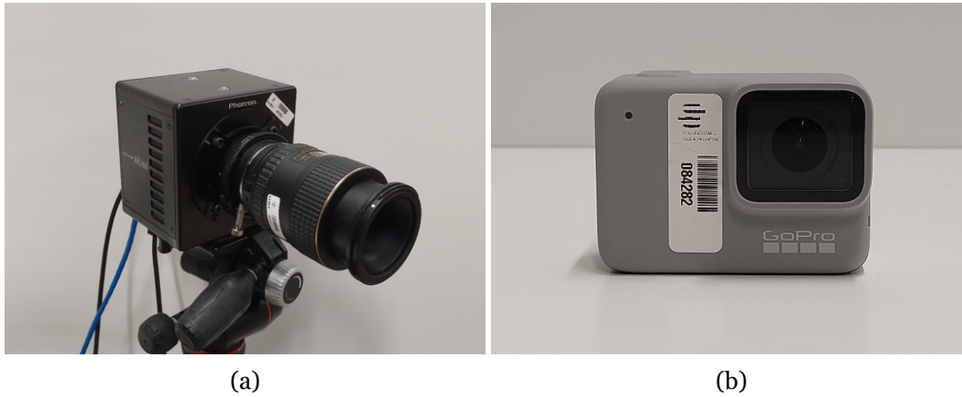
Figure 3.6: Image acquisition systems: a) Photron FASTCAM mini UX50 with a Macro Lens Tokina AT-X M100 AF PRO D; b) GoPro Hero 6.
