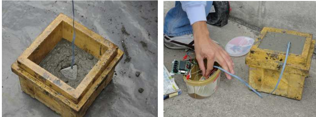
Figure 3.32: Preparations to measure early age concrete temperature and humidity using a SHT21S sensor inside a mortar cube.
