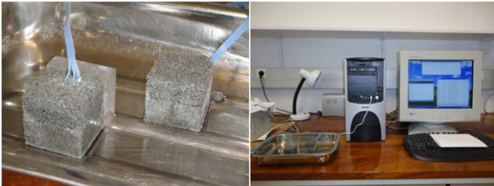
Figure 3.31: Setup to measure temperature and humidity using an SHT15 sensor inside a mortar cube for sensor protection.
