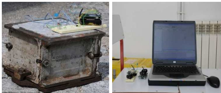
Figure D.1: On-going measurement of temperature with wireless sensors inside a concrete cube.
