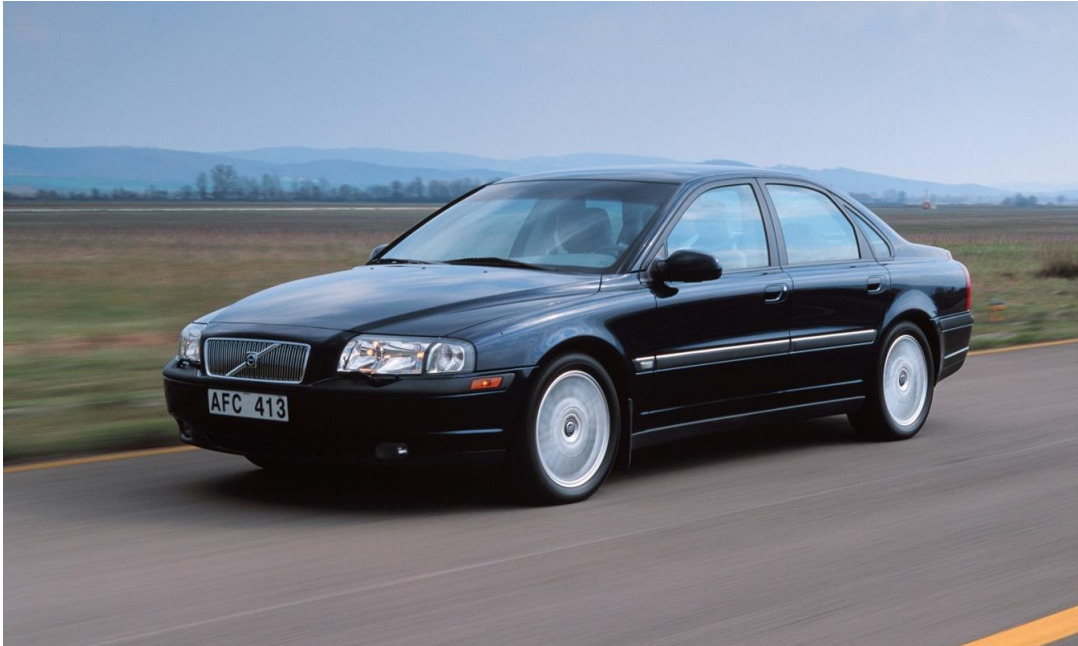
Figure 47: The shoulder line, V-shaped hood, the grille, and soft nose present in the 1998 Volvo S80 (Volvo, 2004).
