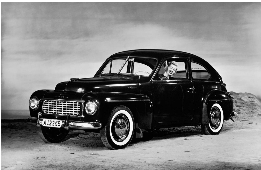
Figure 46: The shoulder line, V-shaped hood, the grille, and soft nose present in the Volvo PV 444 1946-1958 (Volvo, 2002a).
