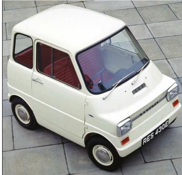
Figure 22: The Comuta prototype, Ford's attempt at an electric city car in the 1960s (Burton, 2013).
