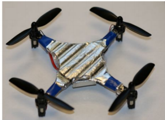
Figure 2.36: Corrugated Zn/MnO 2 battery pack design as a replacement for the original device cover to support UAVs' main power source. Reproduced from [118].
