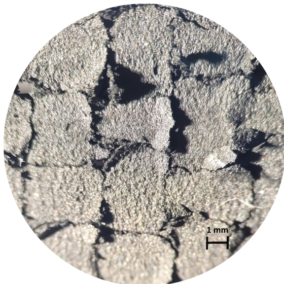
Figure 4.2: (a) Initial state of the graphene coated carbon fiber (b) Final state of the graphene coated carbon fiber after deformation.
