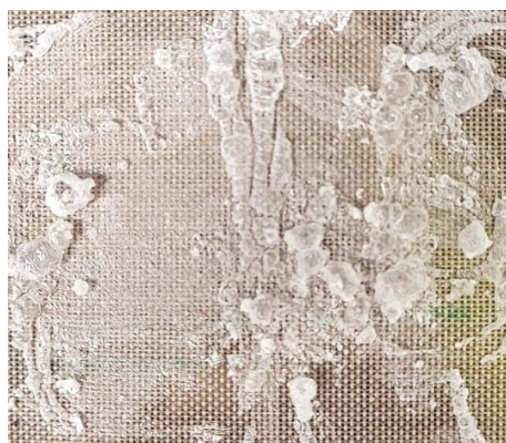
Figure 4.4: Compound formation due to the reaction of the ionic liquid with air.
