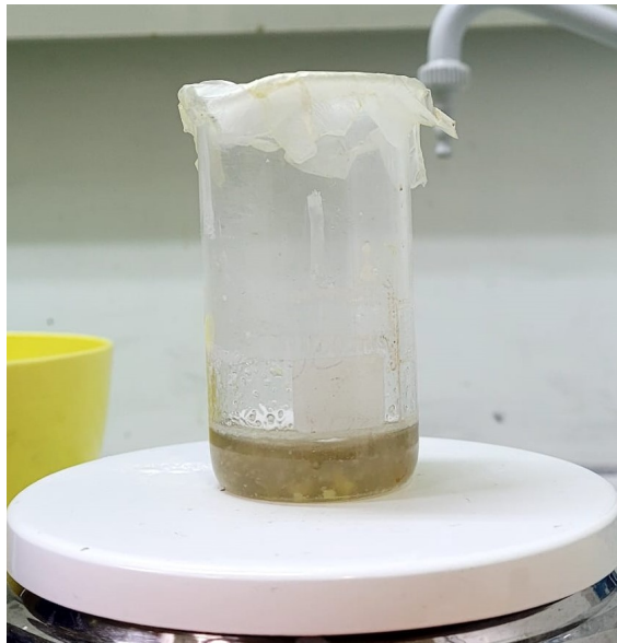
Figure 3.4: Final steps of the manufacture of the ionic liquid, \text{AlCl}_3 -Urea at a molar concentration of 1.4:1.
