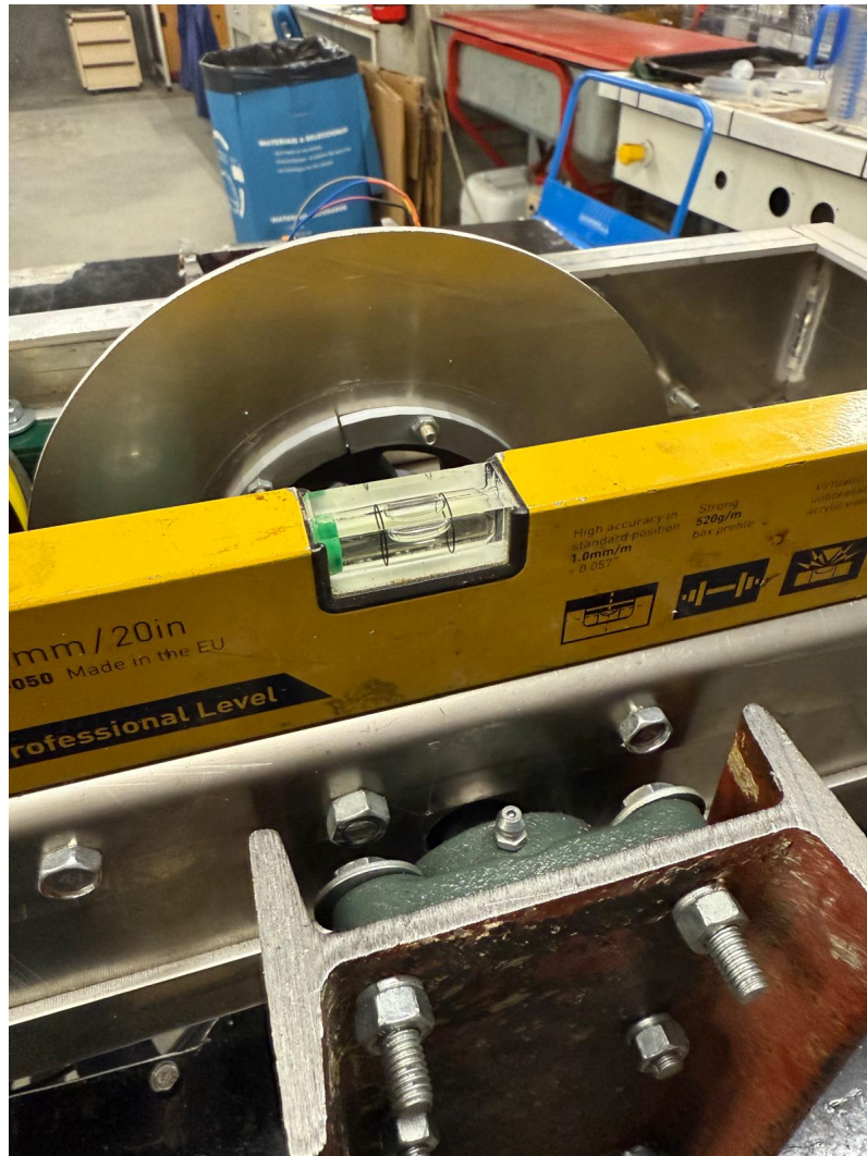
Figure 3.11: Level used to ensure that the structure was perpendicular to the load cell.
