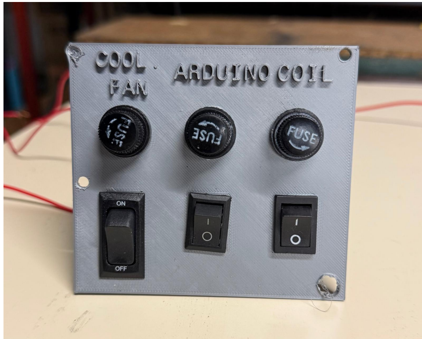
Figure 3.23: 3D printed plate that houses the fuses and switches of the electric system of the ETB.
