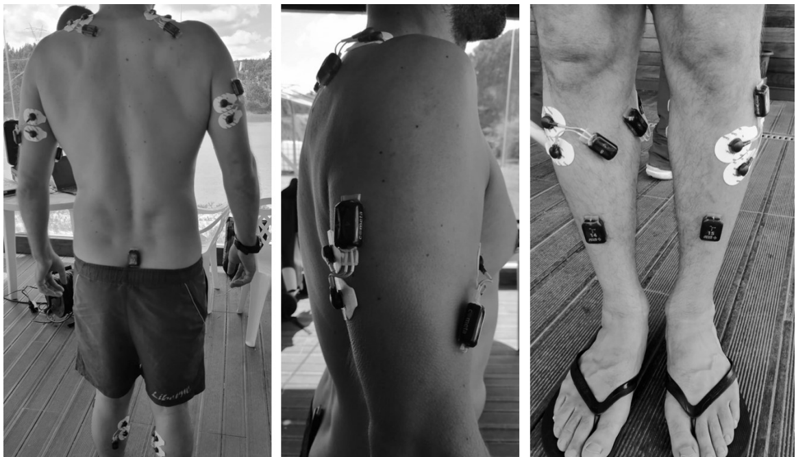
Figure 1. Participant equipped with surface electromyography electrodes.
