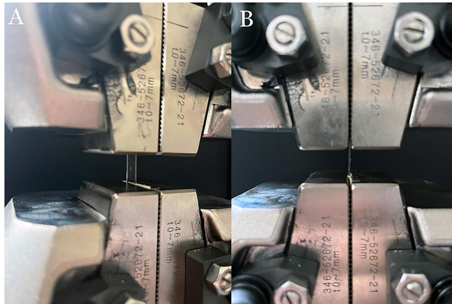
Fig. 49. Placement of PDMS strip samples in the Shimadzu AGS-X universal testing machine: (A) Oblique view; (B) Front view.
