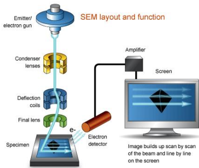
Fig. 53. Main components of a SEM microscope. (Adapted from [100]).
