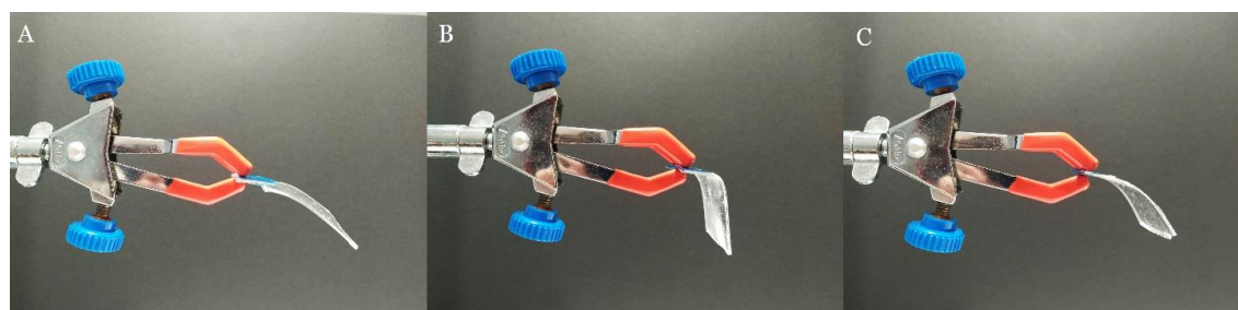
Fig. 40. Self-deflection, under own weight, of different configurations of PDMS elastomer: (A) PDMS@10:1 ratio; (B) PDMS@15:1 ratio; (C) PDMS@20:1 ratio.
