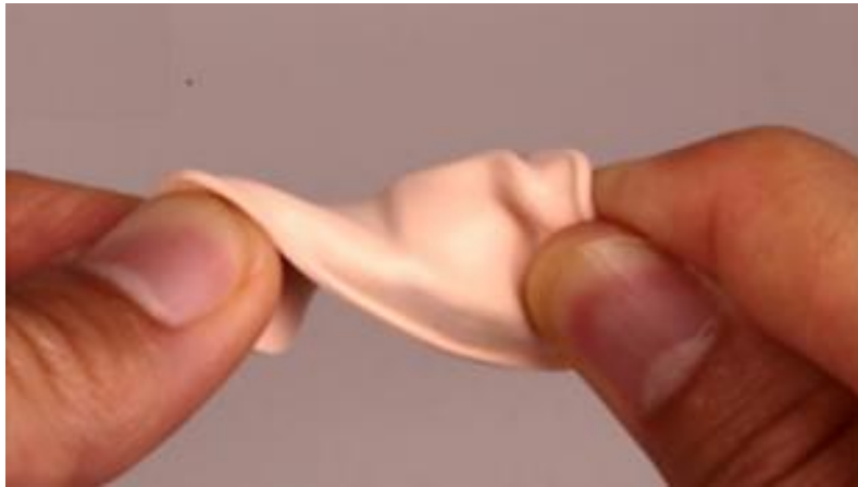
Fig. 14. Mechanical robustness of a throat-worn pressure sensor being evaluated. (Adapted from [33])
