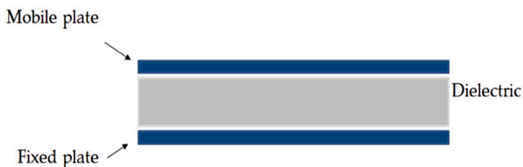
Fig. 20. Capacitive flexible humidity sensor with a parallel plate electrode mechanism. (Adapted from [41])
