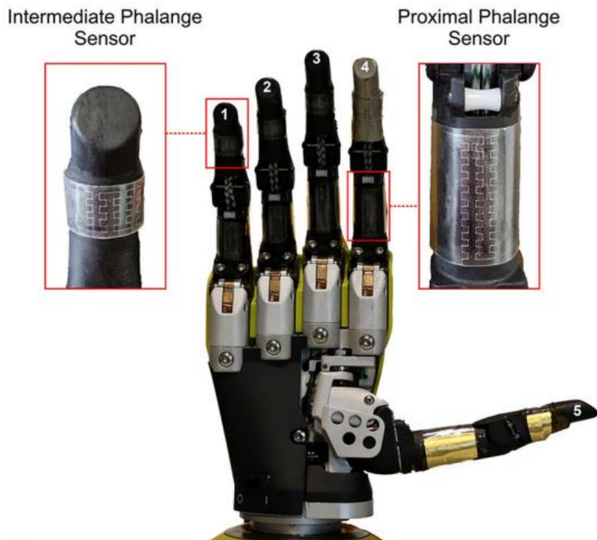
Fig. 27. Sensorial system integrated into a robotic hand. (Adapted from [53])
