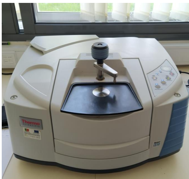
Fig. 55. Nicolet™ iS 10 spectrometer, employed in the ATR/FTIR characterisation of pristine PDMS films and rGO@PDMS composite films.
