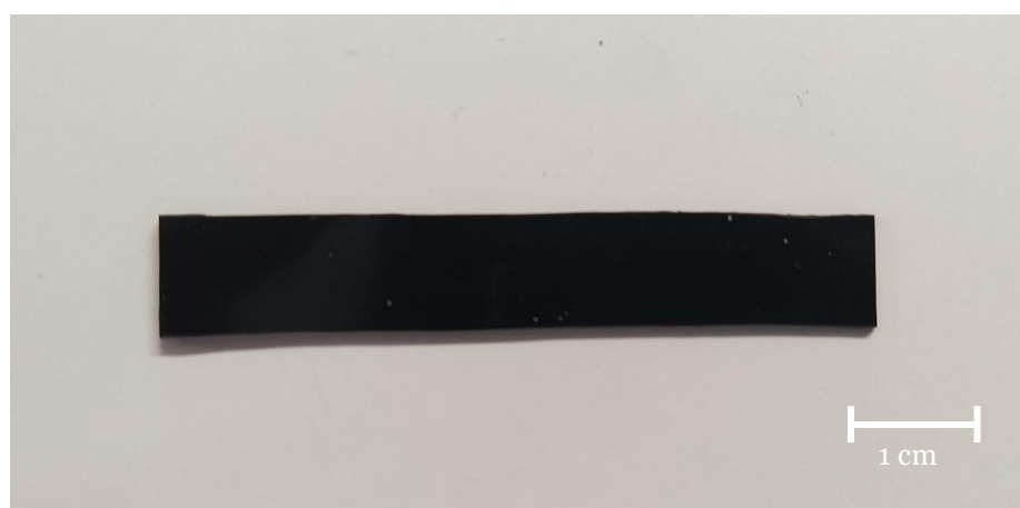
Fig. 52. rGO@PDMS composite sample used during mechanical testing.
