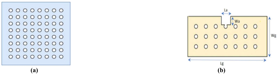
Figure 6. (a) Schematic structure of proposed PhC. (b) proposed microstrip patch array antenna ground configuration.
