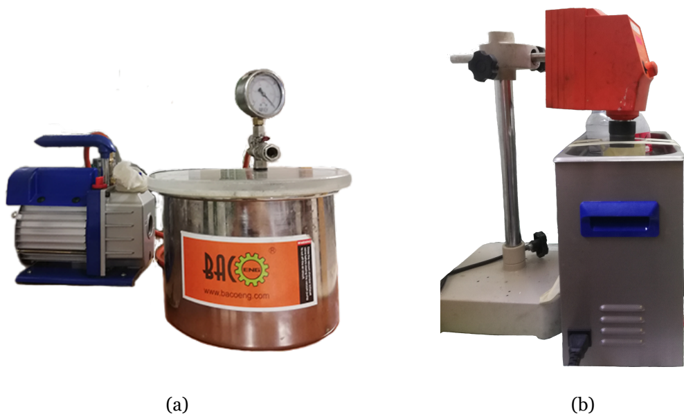
Figure 3.2: (a) Bacoeng vacuum chamber and vacuum pump - VEVOR 3CFM. (b) Digital overhead stirrer LBX OS20 series - vertical rotation stirrer and sonication bath - Ultrasonic Cleaner model AU-65.
