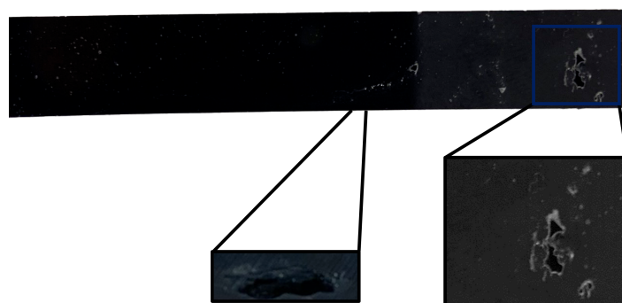
Figure 3.4: Macroscopic observation of nanocomposite defects. Two types of defects are visible - voids (on the surface) and areas with incomplete curing (through-thickness).
