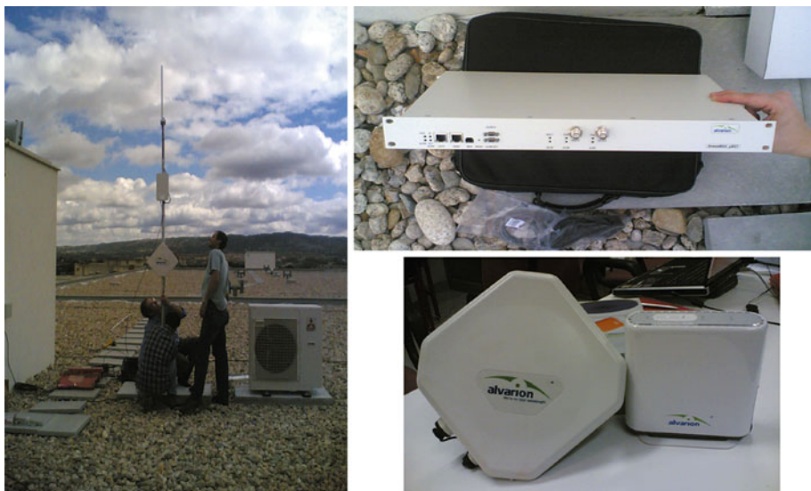
Fig. 1 IEEE 802.16-2004 PtM equipment operating at the experimental setup
