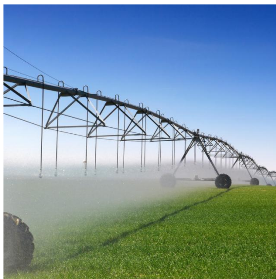
Figure 4. Sprinkler irrigation system (retrieved from Patel & Prajapati, 2020).
