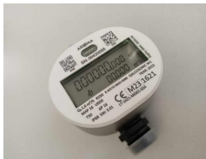
Figure 35. Axioma Qalcosonic W1 smart water meter
