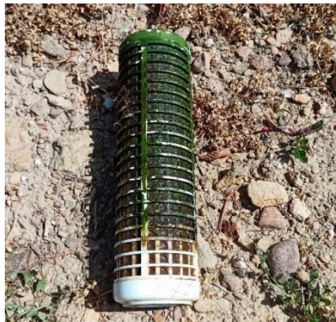
Figure 54. Clogged 50 µm water filter.
