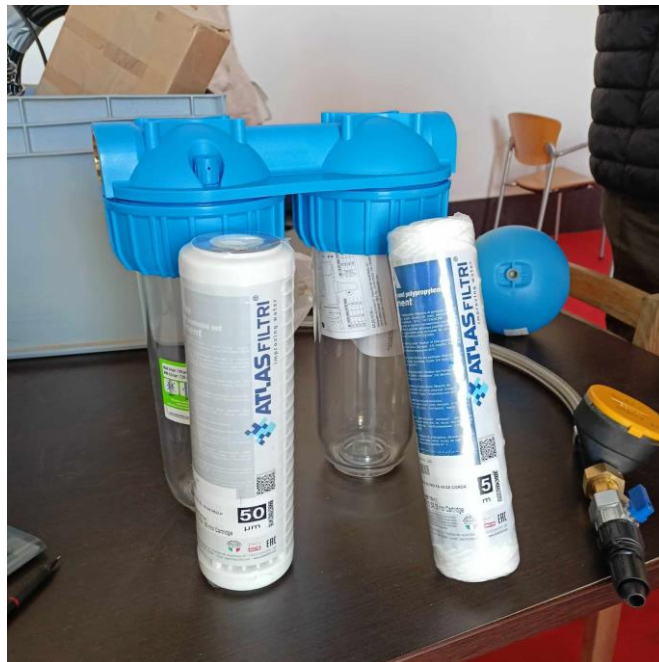
Figure 25. Primary water filtration system before the 1 m 3 water tank, at the Peach Trees field test
