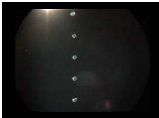
Figure 6.5 Local nodes of an acoustic standing wave made visible by levitation of small water droplets.
