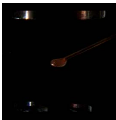
Figure 7. Detaching a droplet from a silicon coated capillary tip.
