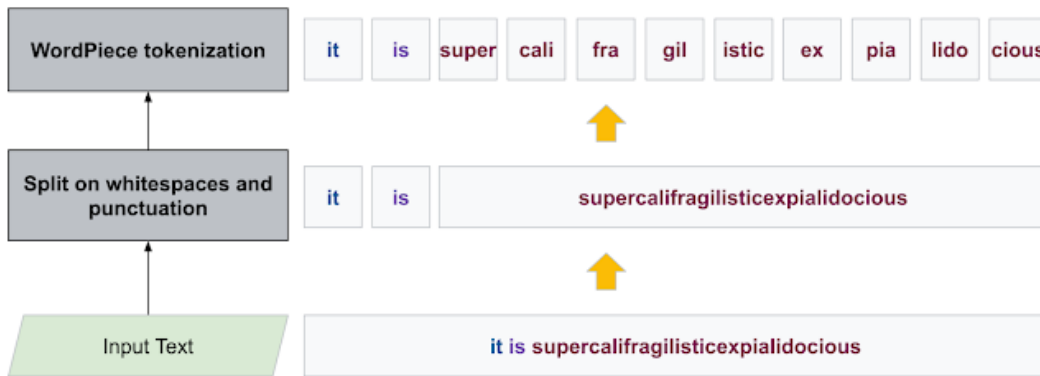
Figure 3.9: The WordPiece tokenization process with an example sentence [6].
