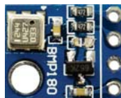
Figure 3.11: Temperature and pressure sensor [64].
