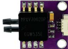
Figure 3.12: Differential pressure sensor [66].
