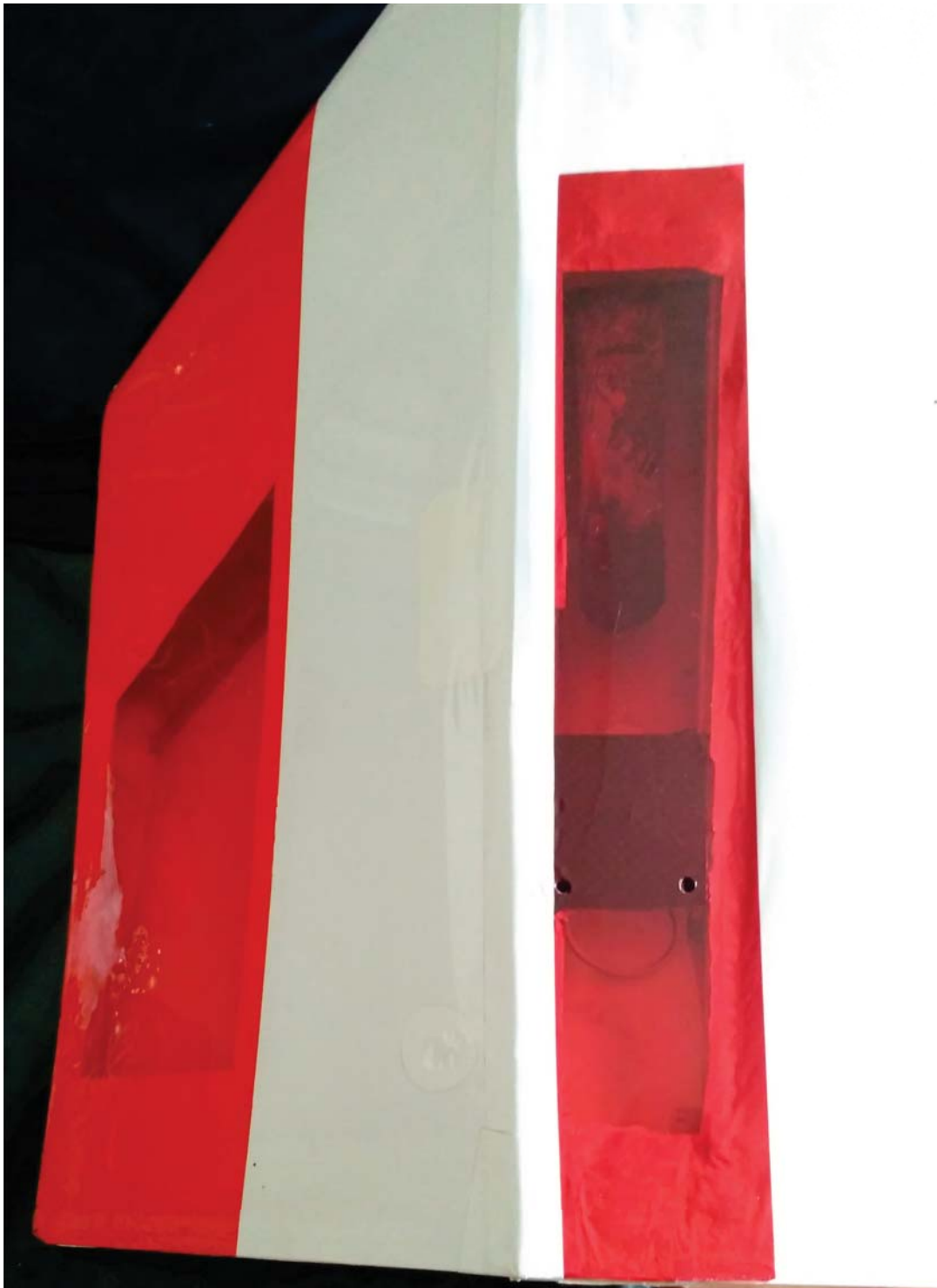
Figure A.3: Wing tip tail tube with hard point to receive the tail surface clamp.
