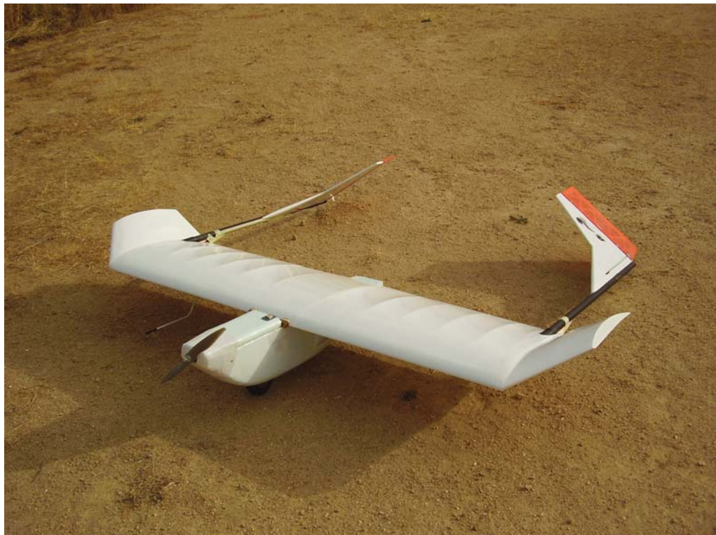
Figure 3.3: Wingtip tail configuration.
