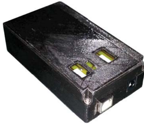
Figure 3.18: 3D printed PLA case for the complete system.
