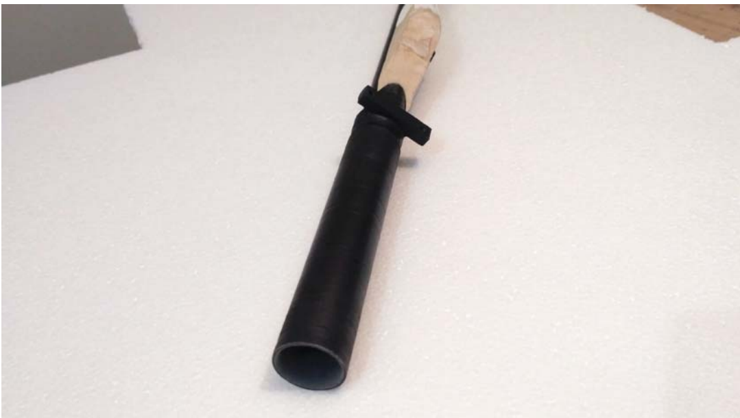
Figure A.2: Tail surface tube with female interface and 3D printed clamp for wing attachment.
