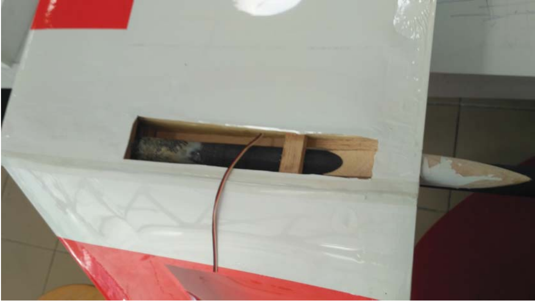
Figure A.1: Wing tip tail tube before the creation of the interface.
