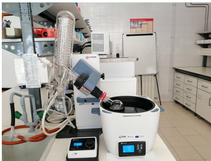
Figure 2.5: Rotary evaporator used for the elimination of the extraction solution.
