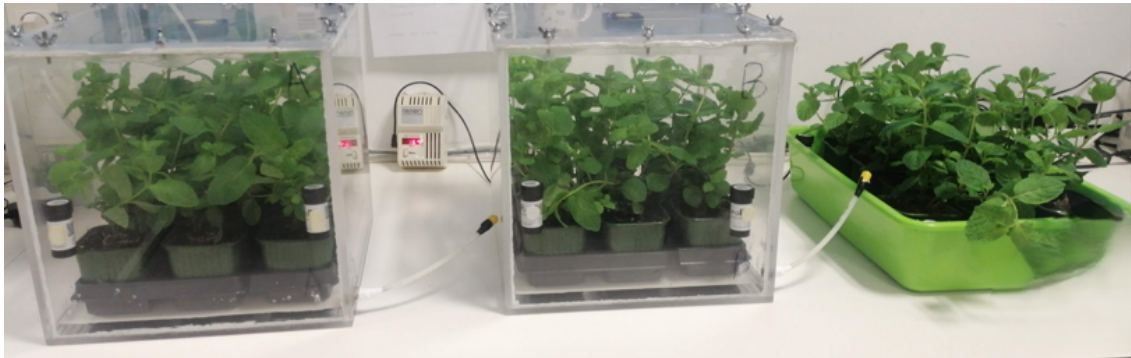
Figure 2.1: Experimental setup showing Mentha spicata plants in Chamber A (right) and B (center) sealed acrylic chambers during the 15-day radon exposure period, and the absolute control, Group C (left). Source: LabExpoRad
