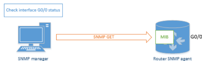
Figure 2.3 - Example of a SNMP GetRequest.
