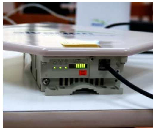
Figure 17: RB LEDs for the received power.
