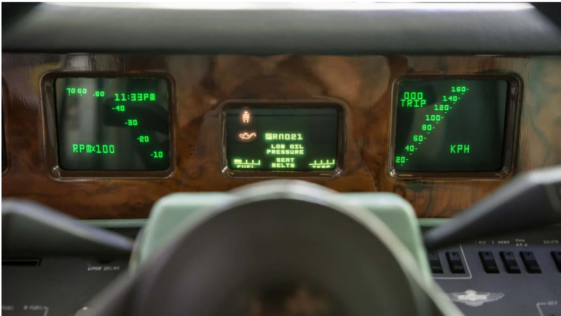
Figura 61 - Painel de instrumentos digital do Aston Martin Lagonda de 1976, (Opposite Lock, s.d.).
