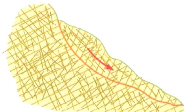
Figure 41. Diagram of a curved failure surface in heavily jointed rock (Vallejo, Ferrer et al., 2004).
