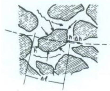
Figure 24. Water pressures on the soil grains as water flows through (Guidicini & Nieble, 1984).
