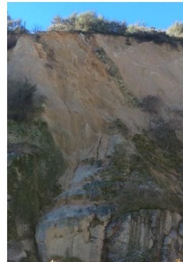
Figure 43. Example of granitic residual soil slope with parent rock visible at the bottom.
