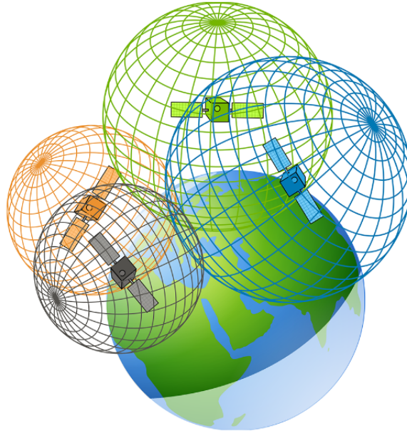
Figure 2.3: Four satellites used for trilateration around a location on Earth. Adapted from GISGeography in “How GPS Receivers Work – Trilateration vs. Triangulation”, 2022[GIS].
