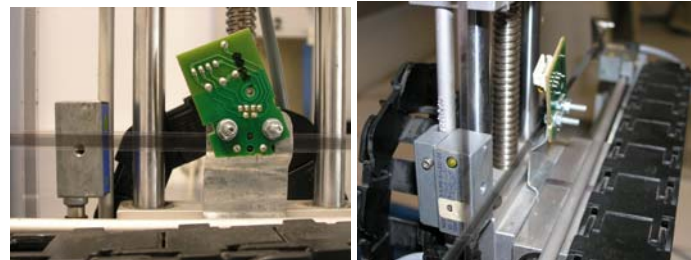
Linear optical sensor for longitudinal movement
