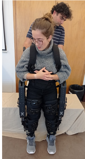
Figure 3.8: Exoskeleton to a sit-to-stand position during the experimental activity.
