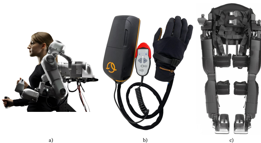
Figure 2.3: Exoskeletons types: a) Harmony exoskeleton produced by ReNeu Robotics Laboratory is an upper body exoskeleton (adapted from [29]); b) Ironhand produced by Bioservo Technologies is an active soft hand exoskeleton (retrieved from [30]); c) REX produced by Rex Bionics is a lower-limb exoskeleton (adapted from [31]).
