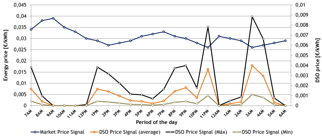
Figure 5.7: Price signals comparison at each DS node in the modified 16-Bus DS.
