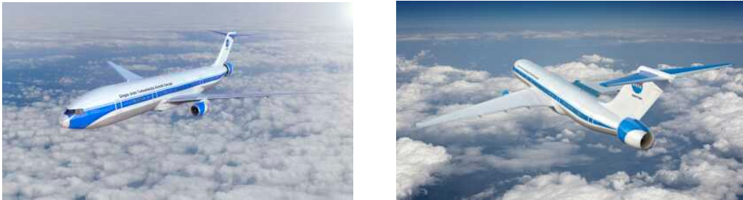
Figure 2.7: NASA Single-Aisle Turboelectric Commercial Transport (STARC-ABL) concept. [10:11]
