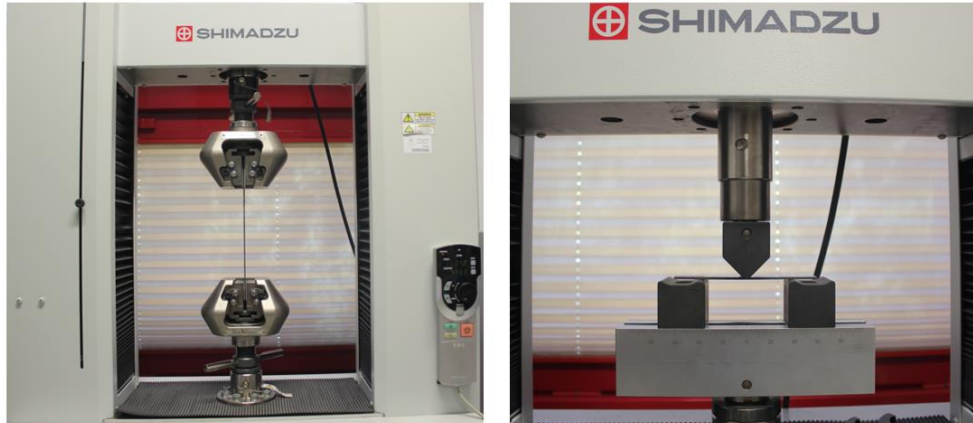
Figure 3.5 – Experimental setup of the tensile (on the left) and flexural (on the right) tests.
