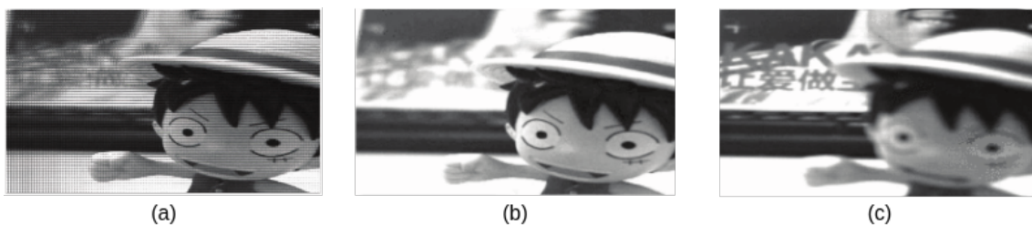
Figure 2.7: The frequency domain refocusing effects [7]. (a) Raw image, (b) and (c) Images refocused at different focal planes: one focused on the background and the other on the foreground.
