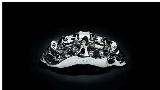
Figure 2.4: Titanium eight-piston monobloc brake caliper produced by additive manufacturing technologies [55].
