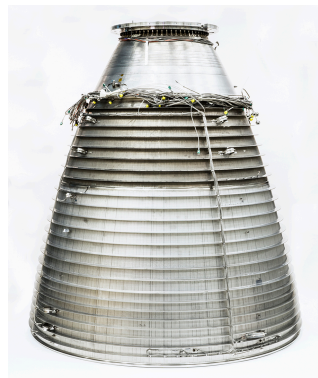
Figure 2.6: Advanced Ariane 6 nozzle (SWAN) to be incorporated in the Vulcan 2.1 engine [60].
