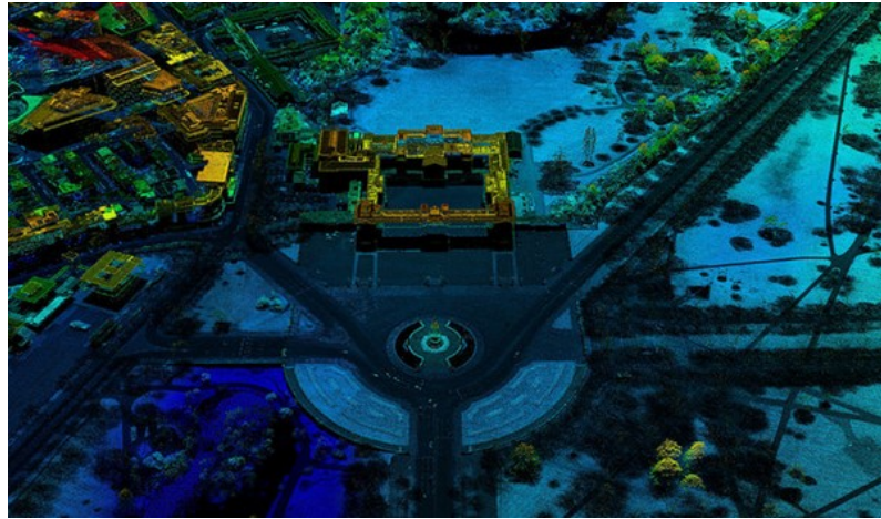
Figure 1.5: An example of a point cloud of wide area scanning. The data is of high resolution, but without accurate material appearance information or color. The color in this figure represents height and is not related to the color of the imaged scene. The image is a LIDAR scan of Buckingham Palace, UK and is courtesy of Environmental Agency ( https://www.flickr.com/photos/environment-agency/27489358013 ) [CC BY 2.0 ( https://creativecommons.org/licenses/by/2.0/ )] (Figure taken from [1]).
