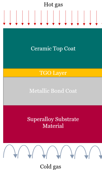
Figure 3.6: Schematic illustration of a traditional TBC system (not to scale).
