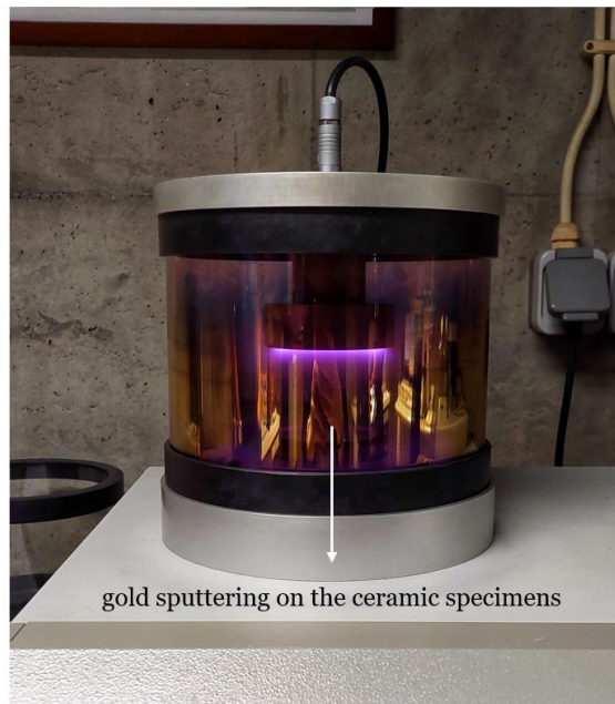
Figure 4.13: Ultra-thin gold coating deposition.
