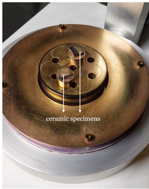
Figure 4.12: Ceramic samples with an ultra-thin gold coating.
