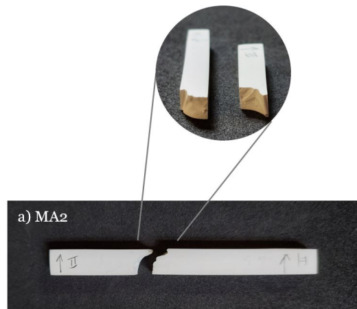
Figure 5.14: Fracture mode geometry of MA2 ceramic composites.
