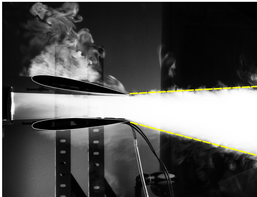
(b) Straight jet flow with plasma actuation on.
