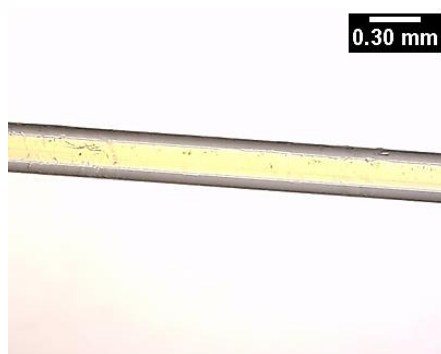
Figure 28 – Images captured 14 days after the Counter Diffusion test, where the initial concentration of the precipitating solution was reduced by half. The observed capillary has a magnification of 30x and as a reference value, the capillary has a diameter of 0.30 mm.
