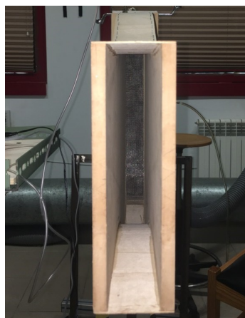
Figure 3.3: Nozzle exit of the contraction developed by ref. [40].
