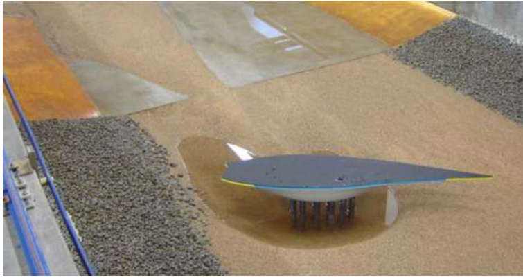
Figure 5.12: Equilibrium state following local scour tests.
