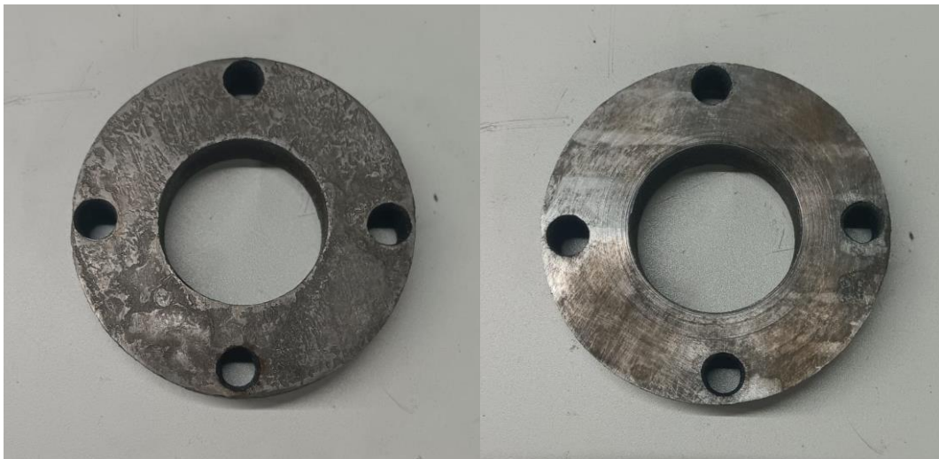
Figure 20 - NF2 after hardening and cleaning processes.
