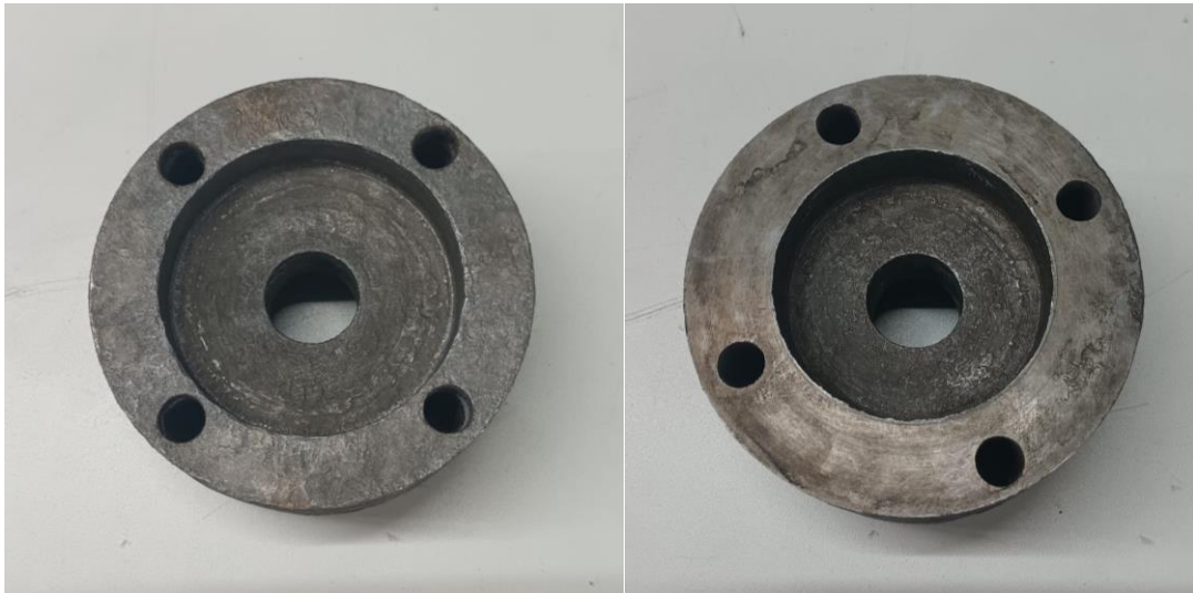
Figure 19 - NF1 after hardening and cleaning processes.
