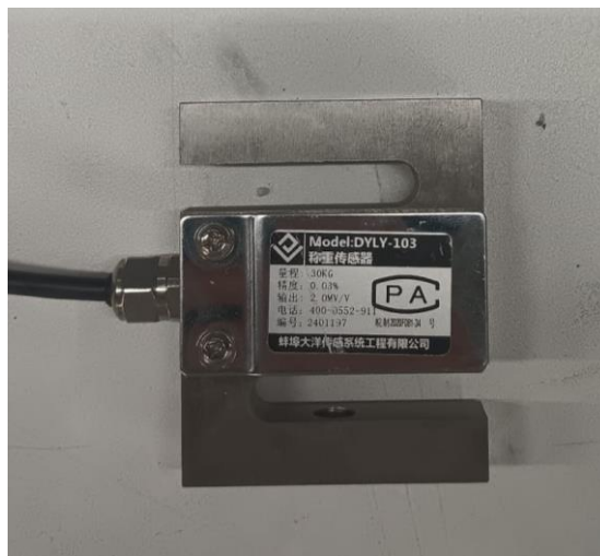
Figure 32 - Load cell used for tank weight readings.
