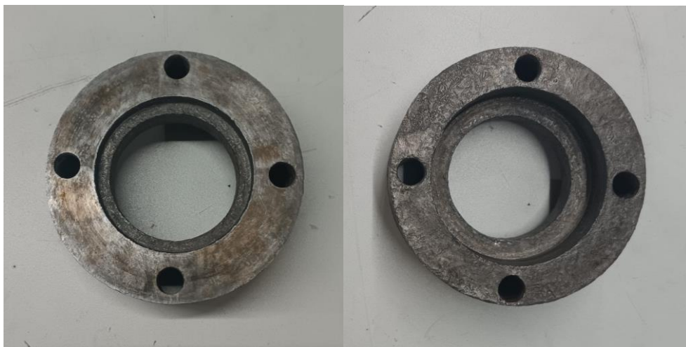
Figure 18 - IF2 after hardening and cleaning processes.
