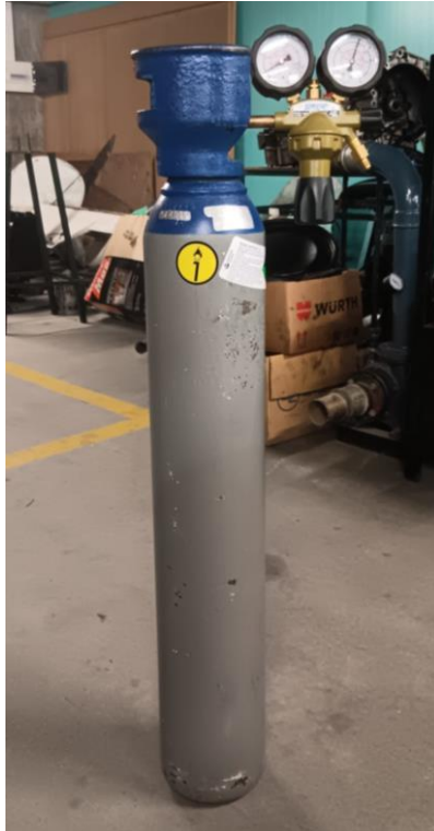
Figure 28 - Nitrous oxide tank coupled with a pressure regulator.
