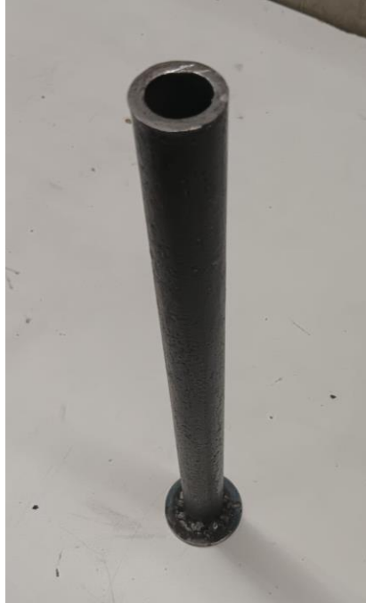
Figure 21 – Component used to create the fuel grain port.
