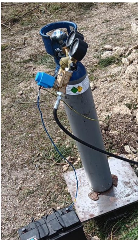
Figure 42 - Nitrous oxide tank with a bend in the feed line.
