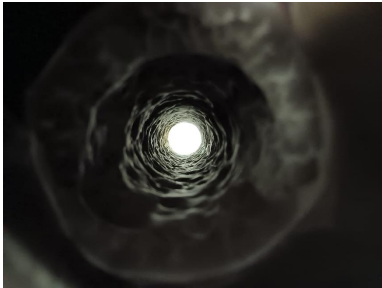
Figure 43 - Paraffin grain port after test 2.
