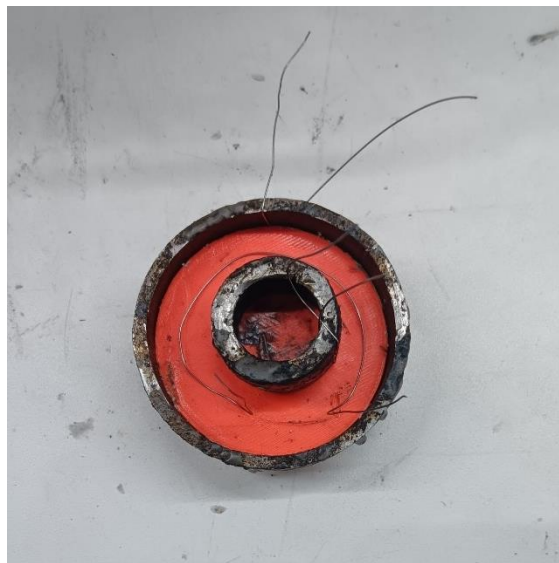
Figure 24 - Charge mould with nichrome wires.
