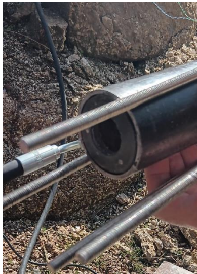
Figure 26 - Charge inside the motor.
