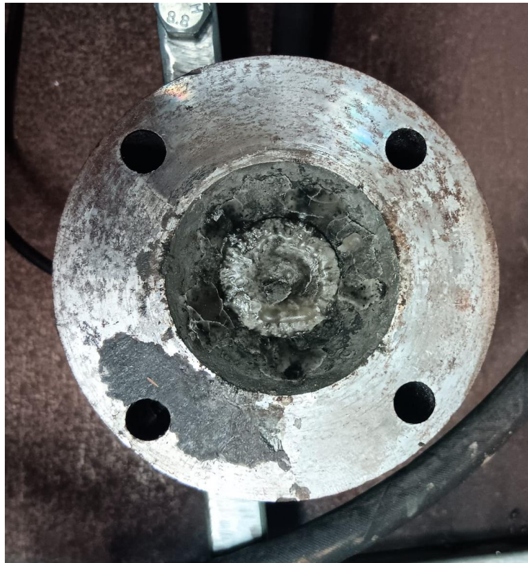
Figure 41 - IF1 after testing shows white bubble-like formations.
