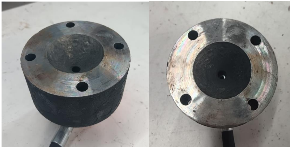
Figure 17 - IF1 after hardening and cleaning processes.
