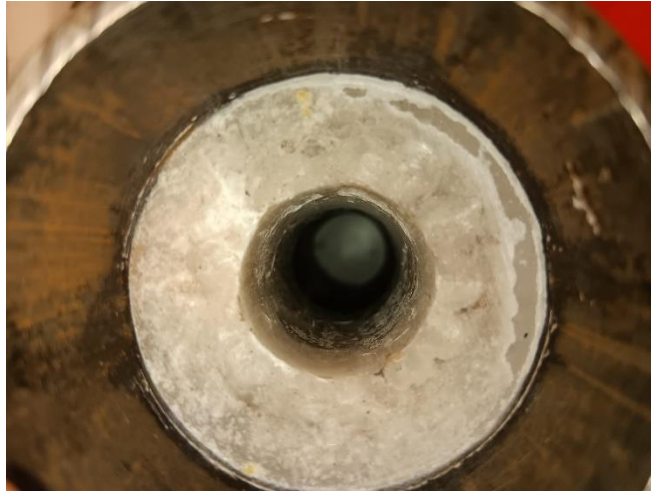
Figure 23 - Solidified fuel grain inside the combustion chamber.
