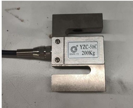
Figure 31 - Load cell used for traction readings.
